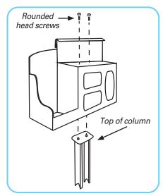
4. To mount the station, place station on top of column. Use included Allen Wrench to secure station to column with (2x) rounded head screws.
