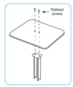
2. Use included Allen Wrench to secure base to column with (2x) flathead screws.
