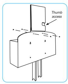
5. To mount the sign holder, align the holes of the holder with the holes at the top of the station. Thumb access to printed sign faces back of station.
